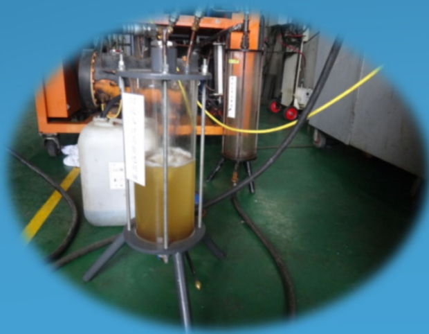
Polluted refrigerant before reclaiming process
