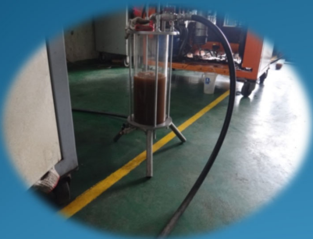
Polluted refrigerant before reclaiming process
